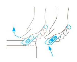
Following cutting, the blade immediately retracts into the handle. Condition: you have **released hold of the slider**.
